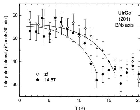
Fig. 1: Temperature dependence of the integrated intensity of the (201) reflection measured on E4
