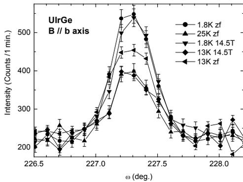
Fig.2: (201) reflection measured at E4 at various thermodynamic conditions.
