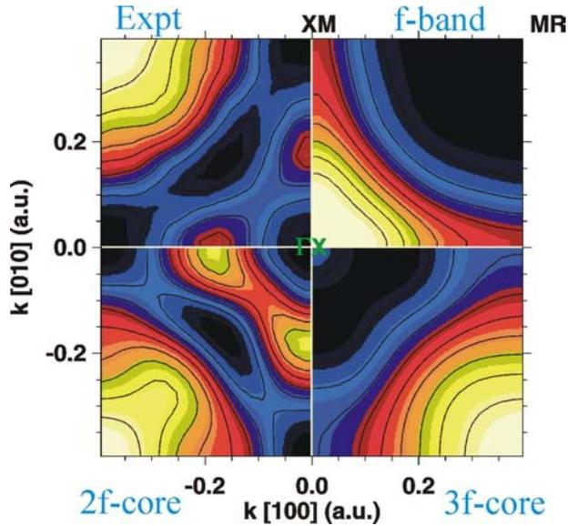
Figure 2: Projections of experimental (left top) and calculated Fermi surfaces of  $\text{UGa}_3$ . Top right displays results for 5f in band calculation, bottom right is from standard open-core calculation and bottom left corresponds to calculations with two 5f electrons treated as localized core states
