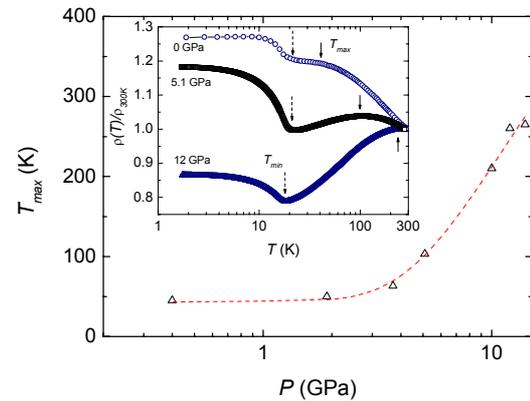
Fig. 1 Pressure dependence of  $T_{max}$ . The inset shows  $\rho(T)/r_{300K}$  as a function of  $T$  at selected pressures.
