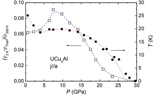
Fig. 2 Pressure dependence of the Néel temperature and the ratio  $(\rho_{2K} - \rho_{Tmin})/\rho_{300K}$ .
