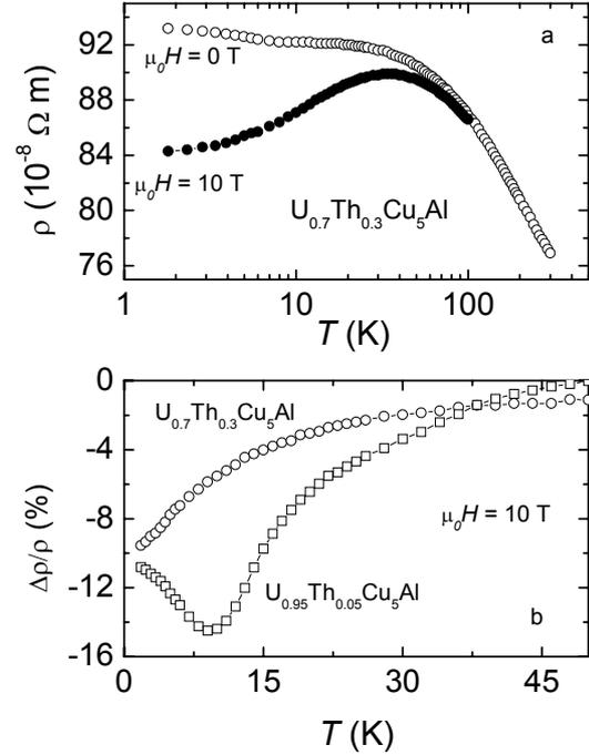
Fig. 3 (a) Temperature dependence of the resistivity of  $\text{U}_{0.7}\text{Th}_{0.3}\text{Cu}_5\text{Al}$ , measured at zero and 10 T. (b) Magnetoresistance of  $\text{U}_{0.95}\text{Th}_{0.05}\text{Cu}_5\text{Al}$  and  $\text{U}_{0.7}\text{Th}_{0.3}\text{Cu}_5\text{Al}$  as a function of temperature.
