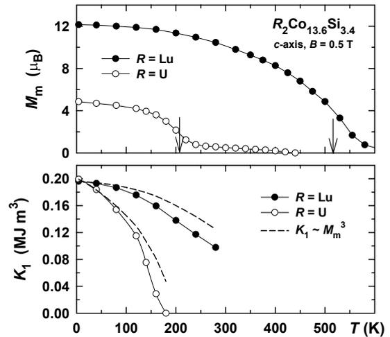
Fig. 2. Temperature dependences of  $M_m$  and  $K_1$  of the  $R_2Co_{13.6}Si_{3.4}$  single crystals. The arrows indicate  $T_C$ .
