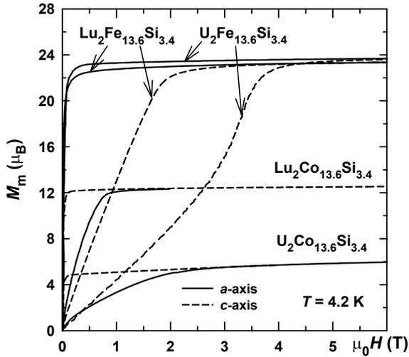
Fig. 1. Magnetization curves along the main axes of the  $R_2T_{13.6}Si_{3.4}$  single crystals.
