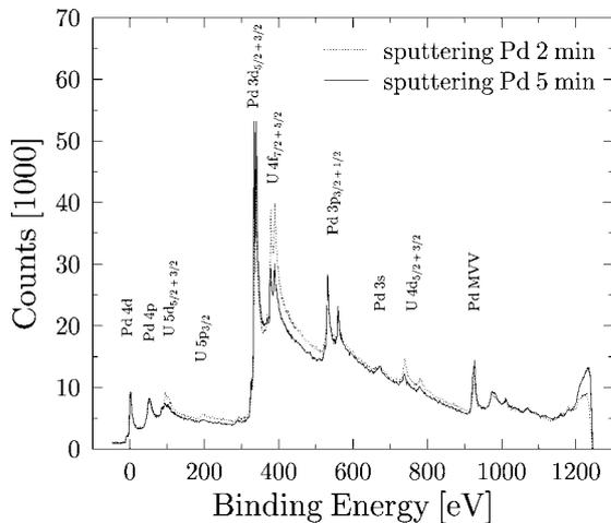
Fig. 1. XPS spectrum for the growth of a Pd capping layer onto a uranium film.
