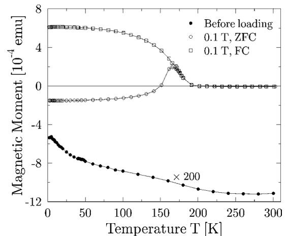
Fig. 2. Magnetisation as a function of temperature before (lower part, multiplied by 200) and after H-loading (upper part) for 1 hour under 1 bar atmosphere.
